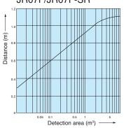
Distance-output Characteristics (Typical Example) JT10R/JT10R-SR JRM3R/JRM3R-SR JT10RF/JT10RF-SR
